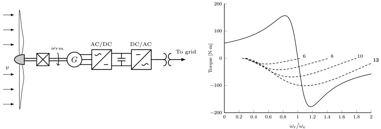
Fig. 1: (left) notional wind turbine system, (right) generator electromagnetic torque (solid), and mechanical torque (dashed) for wind velocities  $v \in \{6, 8, 10, 12\}$  [m/s].
